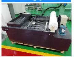
The cooling system is designed with double oil tanks. The rolling oil is filtered precisely and the filter paper can only be reeled. Forced water cooling technology can effectively suppress the temperature rise of rolls and ensure rolling accuracy.
